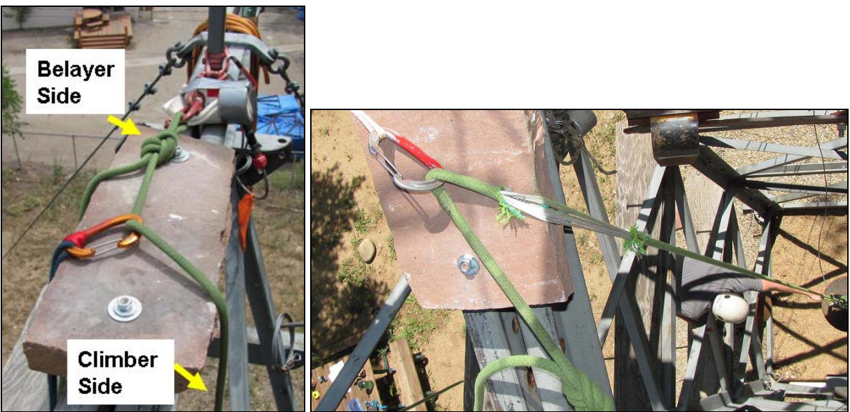
Figure 9. a) Example pre-drop configuration. b) Typical partial rope failure result.
