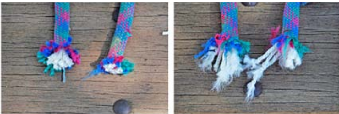
Figure 8. a) Tensioned rope cut with a sharp knife. b) Tensioned rope cut with a sharp rock.
